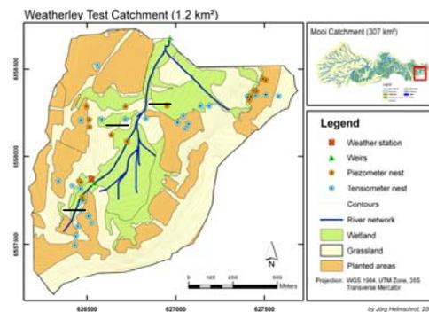
**Figure 1.** Characteristics and instrumentations of test catchment Weatherley
