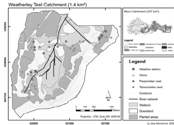
Figure 1. Instrumentation and characteristics of test catchment Weatherley and Mooi basin.
